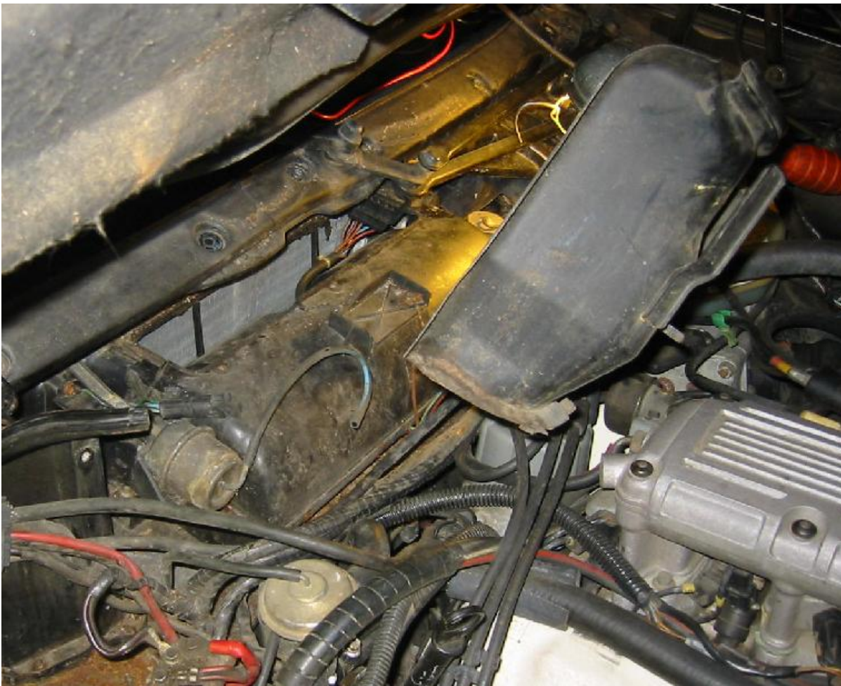
This shows the cuts to be made in the case. The plastic is rather flimsy. After cutting, there are several clips holding the top and bottom halves together that need to be removed.
